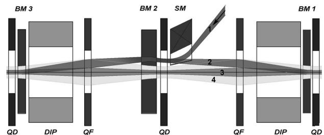
Figure 4: Injection system layout and beam orbits and envelopes: 1 – injected beam, 2 – ‘bumped’ one, 3 – circulated beam after first turn injection, 4 – after accumulation; BM 1 ÷ 3 – magnets for the bump formation, SM – injection septum magnet.
