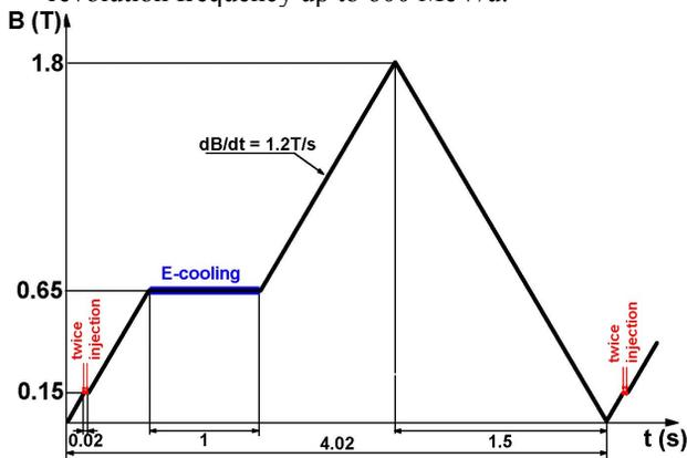
Figure 2: Booster cycle diagram, time is in seconds
