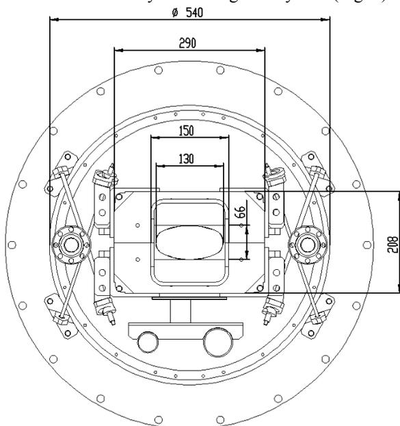
Figure 5: Cross-section of the dipole magnet in cryostat.
