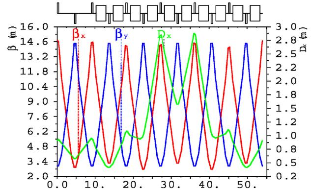
Figure 3: Betatron and dispersion functions for one SP.
