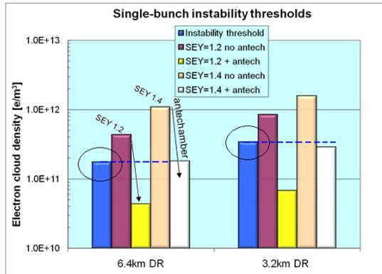
Figure 6 Simulated instability thresholds (blue) in the 6 and 3 km rings compared to the equilibrium cloud density for peak secondary yields  $\delta_{max}=1.4$  and 1.2 with (98% photon absorption) and without (0%) an antechamber. The cloud density is the central near-beam cloud density.
