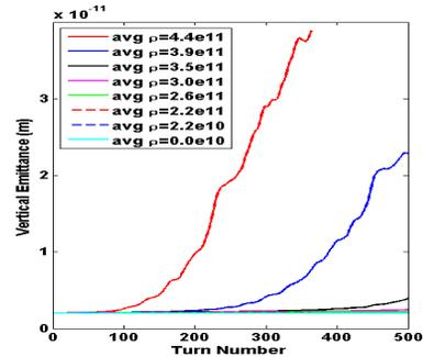
Figure 5: Beam emittance in DSB3 lattice with different cloud densities. The instability threshold is at  $3.5 \times 10^{11}$  e/m<sup>3</sup> according to CMAD simulation.
