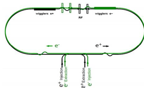
Figure 1: Layout of the ILC damping rings.
