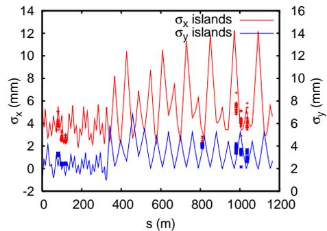
Figure 2: Horizontal and vertical beam rms size at the screens and from the fit.
