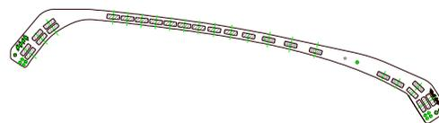
Figure 2: Pole Face Windings.
