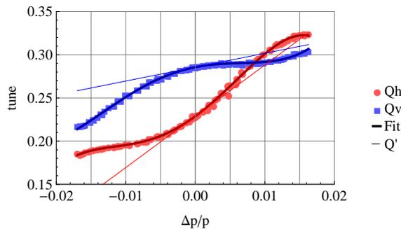
Figure 3: Example of chromaticity determination from tune measurements.
