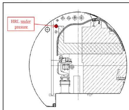
Figure 1: transverse cross section at point 7 – Helium Ring Line under pressure
