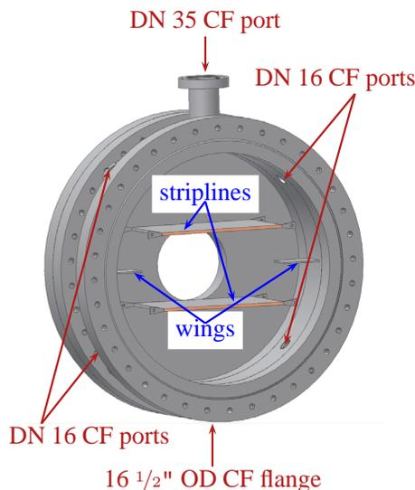
Figure 7: Design of the new spin flip cavity.
