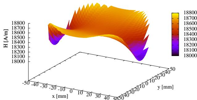
Figure 5: Distribution of the field over the aperture plane perpendicular to the beam.
