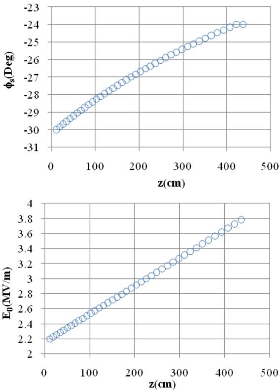
Figure 2: Phase (top) and average axial electric field (bottom) of the DTL.
