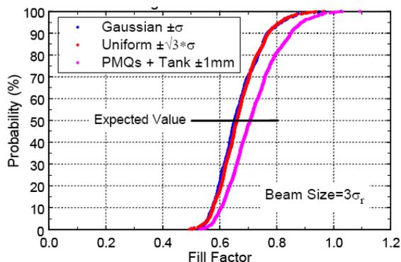
Figure 5: Fill factor analyze with alignment error.
