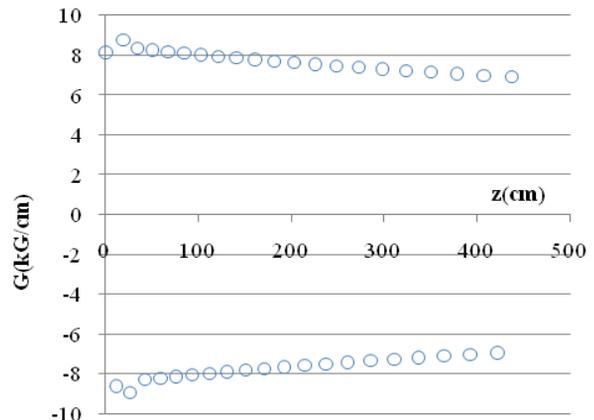
Figure 3: Gradient of the PMQs in the DTL.
