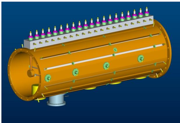
Figure 6: First section model of CPHS DTL cavity.
