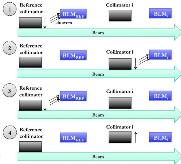
Figure 1: The four-stage beam-based alignment procedure for collimator  $i$ . The reference collimator is aligned to form a reference cut in the beam halo (1). Collimator  $i$  is aligned (2), followed by a re-alignment of the reference collimator (3). Finally, collimator  $i$  is opened to its position in the hierarchy (4).
