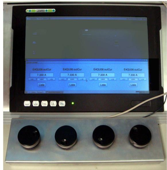
Figure 5: A prototype of the rotary knob user interface. An industrial touch-screen PC runs a Qt-based application. Four rotary knobs are connected to an in-house developed interface board which is in turn attached to the PC by USB.
