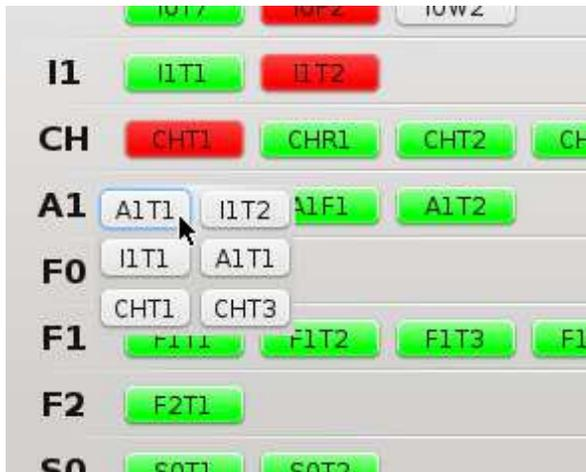
Figure 3: One of the GUI applications which is still to be migrated to an EPICS compatible implementation. The color of each button corresponds to the state of the target screen (red meaning beam is blocked). Left click on a colored button toggles the target's state. Right click will open the subwindow as can be seen on the left. It provides multiple buttons, each representing one of the video multiplexers channels connected to monitors in the control room.
