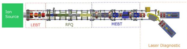
Figure 1: Layout of the Front End Test Stand.
