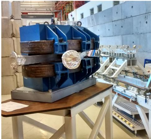
Figure 2: Picture of the existing dipole that can be used for the laserwire beam line.
