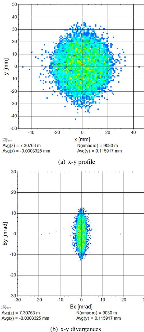
Figure 8: Beam at the entrance face of dump 1.
