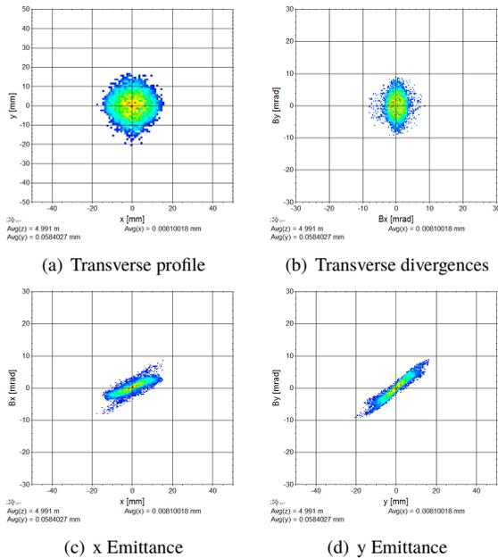
Figure 11: Phase space distribution of the stripped beam used as the input beam for tracking neutrals to the detector.
