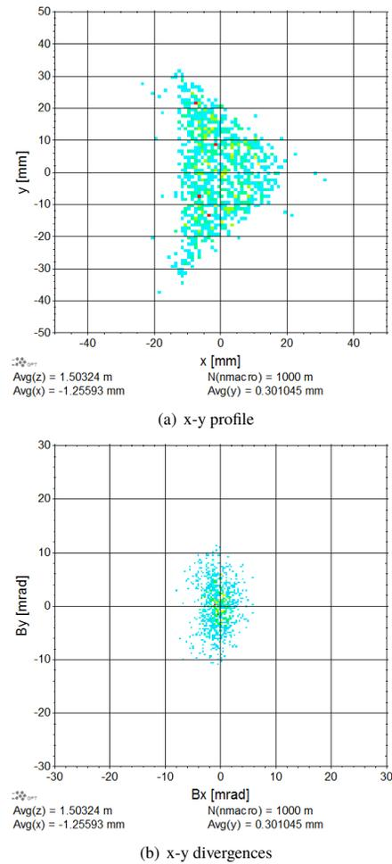
Figure 10: Beam at the entrance face of dump 2.
