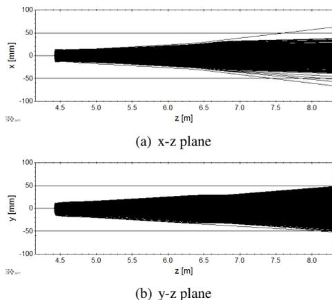
Figure 7: Particle trajectories with the dipole switched off.
