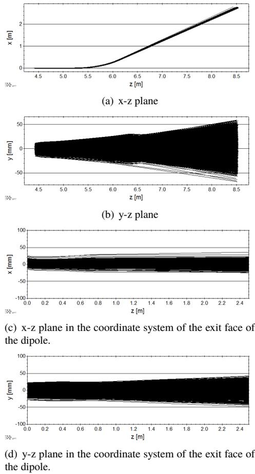
Figure 9: Particle trajectories with the dipole switched on.
