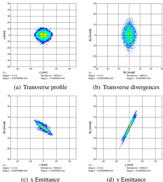
Figure 6: Phase space distribution of the input beam used in the tracking simulations.
