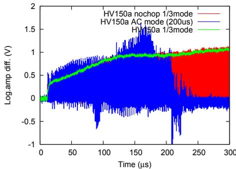
Figure 4: A Log-amp difference output is compared with “1/3 mode” (red: chopped, green: un-chopped,  $500 \mu\text{s}$  injection) and normal circulation mode (blue,  $200 \mu\text{s}$ ).
