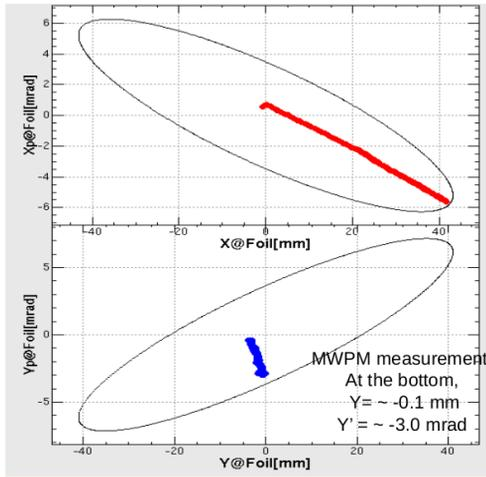
Figure 3: An injection beam footprint on the phase space. It is easy to compare with the desired emittance and painting.
