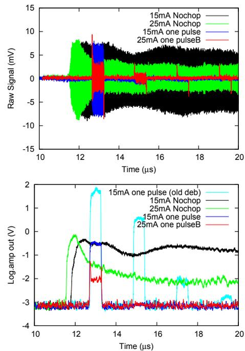
Figure 6: The direct raw signal from the electrode (upper) and 324 MHz Log-amp output (lower) with various Linac beam conditions. Raw data plot of “old debuncher setting” is not shown, but it is about  $\pm 30$  mV.
