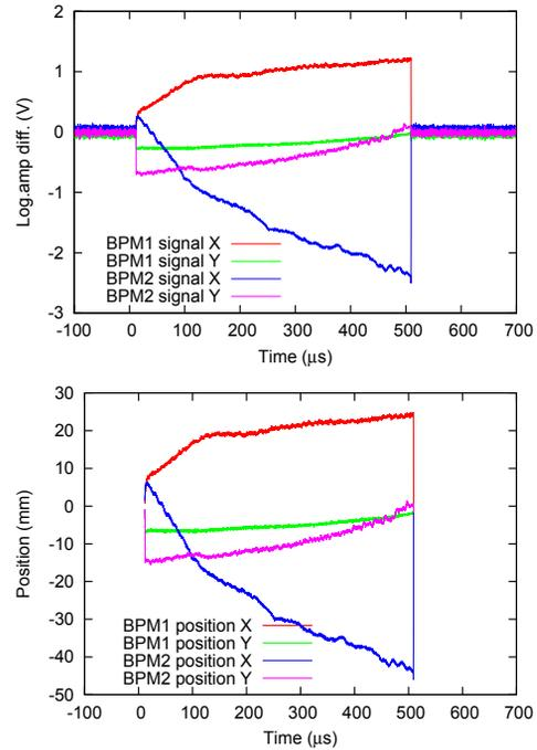
Figure 1: Log-amp difference signal output (upper) and converted position (lower) versus time. The beam was unchopped beam.
