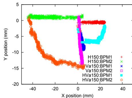
Figure 2: Two BPM X versus Y during 500  $\mu$ s injection period with various painting conditions. “H150” means only horizontal painting with 150  $\pi$ mm-mrad emittance.
