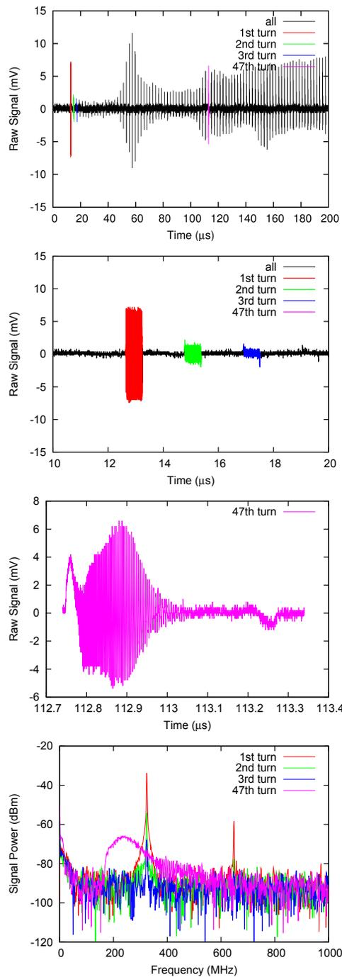
Figure 5: Top is a time domain signal of one intermediate pulse (560 ns). A sampling speed is 5 GS/s. Second and third are its enlargement. The bottom is the FFT spectrum (4096 samples) of specific turn.
