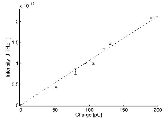
Figure 2: Spectral intensity versus charge at 667 THz of incoherent spectra. The dashed line guides the eye to a linear fit of the data. The errorbars show the standard error. Bunch charge was reduced using scrapers in the bunch compressor.
