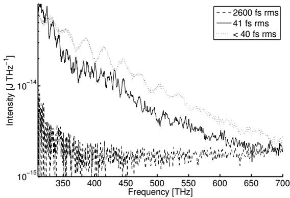
Figure 3: Spectral response, intensity versus frequency, of three different bunch lengths. Single spectrum.
