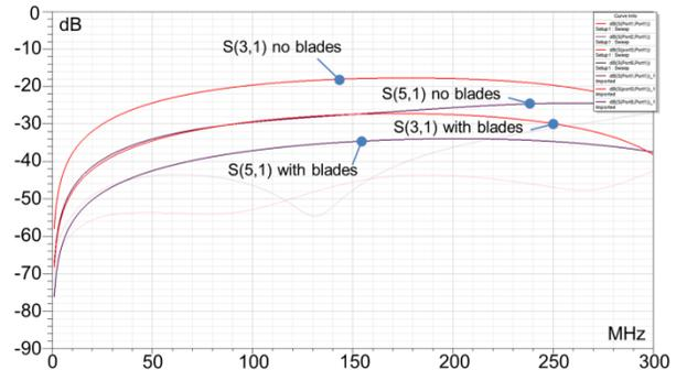
Figure 5: The blades give a -10db improvement in the decoupling of the electrodes. S(3,1) refers to the top electrode in fig 4 and S(5,1) to the left electrode.
