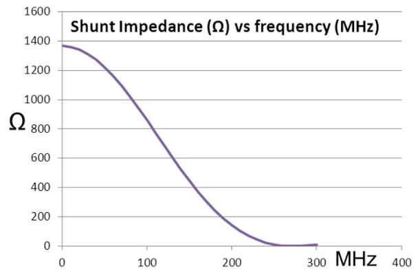
Figure 9: Shunt impedance verses frequency.
