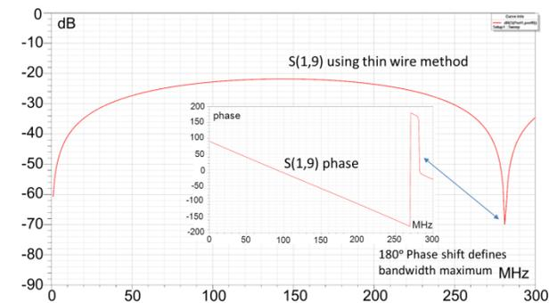
Figure 10: Thin wire measurement of bandwidth.
