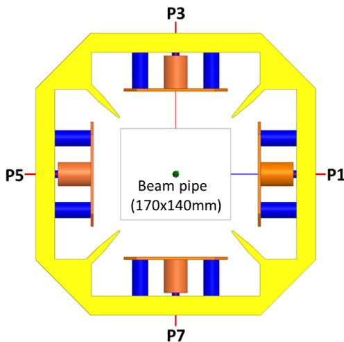
Figure 4: Cross section of the strip line monitor. Note the angled blades that reduce electrode coupling by -10db.
