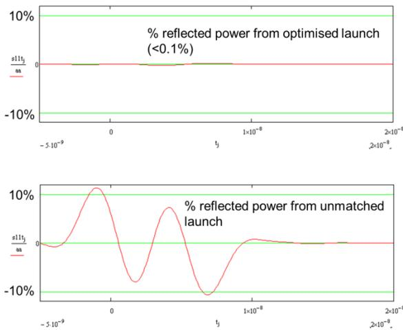
Figure 8: time domain reflections at port 1 showing optimised launch (top) against general launch (bottom) which although mechanically suitable gives a power reflection of 11%.
