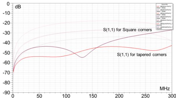
Figure 3: S(1,1) when removing corners of the electrodes to compensate for the capacitance of the PEEK supports.
