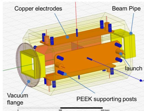
Figure 2: HFSS model of the ISIS strip line monitor showing the copper electrodes, the PEEK supports and the launches used to provide a matched RF path between the feed through and the electrode. The overall size of the monitor is 850 mm long by 425mm wide.
