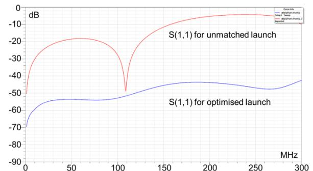
Figure 6: S(1,1) red trace is for a launch mechanically designed only to secure the feed through electrode. S(1,1) blue trace for the fully optimised launch.
