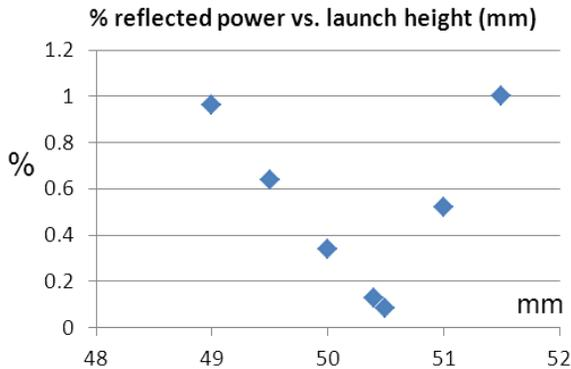
Figure 7: The final tuning of launch height. The y axis is % reflected power and the x axis the launch height in mm.
