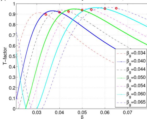
Figure 1: Transit-time factor of different IH structures (defined by  $\beta_g$ ) versus beam velocity  $\beta$ .
