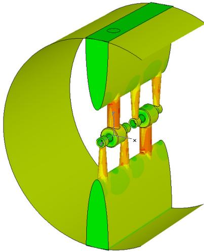
Figure 2: Surface current magnitude in the modified IH1-3 structure (the cavity wall is partially cut).
