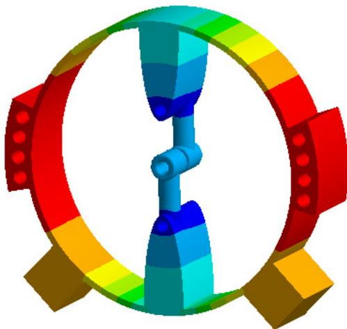
Figure 3: Temperature distribution in regular IH structure.
