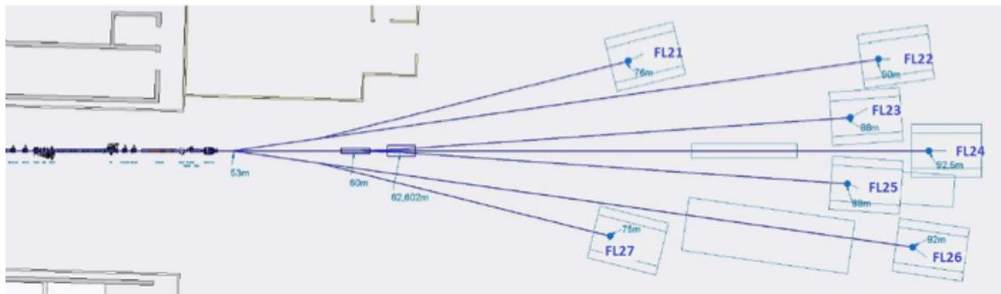
Figure 2: A preliminary FLASH2 beamline distribution with a 14 m main photon diagnostics line and 7 possible beamlines.
