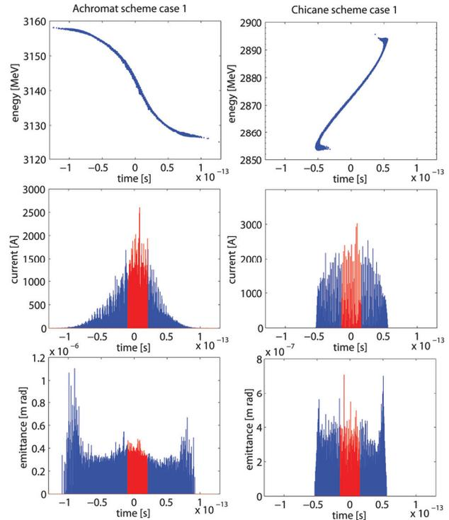
Figure 3: Case 1: Longitudinal phase space(upper-row), slice current(middle-row) and slice emittance(lower-row) of the achromat scheme(left) and chicane scheme(right)
