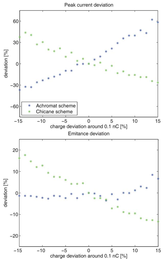
Figure 5: Deviation of peak current(top) and emittance(bottom) due to charge jitter
