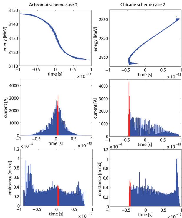
Figure 4: Case 2: Longitudinal phase space(upper-row), slice current(middle-row) and slice emittance(lower-row) of the achromat scheme(left) and chicane scheme(right)
