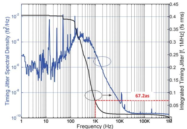
Figure 3: Measured timing jitter spectral density for an individual laser and its integrated timing jitter for the frequency range [f, 1 MHz].
