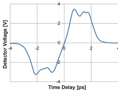
Figure 4: BOC voltage response as a function of pulse time delay.
