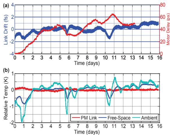
Figure 2: Long-term measurements for the timing-stabilized 1.2-km PM fiber link over 16 days; (a) link drift, as measured by the out-of-loop BOC, and time delay, as controlled by the in-loop motor stage; (b) relative changes in the internal temperatures for the PM link and free-space enclosures and ambient temperature.
