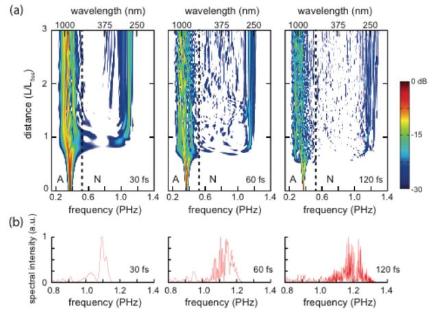
Figure 3: Influence of the input pulse duration with  $t_0/N=0.2$ . Spectrum of the UV band is dramatically degraded as the input pulse duration increases.
