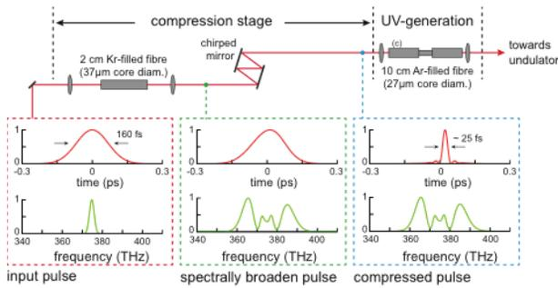
Figure 4: Two stage set-up. The compression stage consists of 2 cm of Kr-filled kagome fibre with 37 µm core diameter followed by a pair of chirped mirrors. Graphs are simulated from a perfect sech-pulse at the input of the compression scheme.
