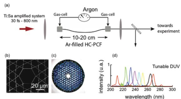
Figure 1: (a) Experimental set-up for the generation of tunable UV light. (b) A scanning electron micrograph and (c) an optical microscopograph of the kagomé-fibre. (d) Tunable UV generated with various combinations of pressure/input power. Each colour corresponds to a different spectrum.
