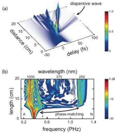
Figure 2: Temporal and spectral evolution of a  $1.5 \mu\text{J}$  30 fs Gaussian pulse propagating inside 20 cm of kagome-fibre filled with 10 bar of argon gas. The dispersive wave is generated after  $\sim 6$  cm.
