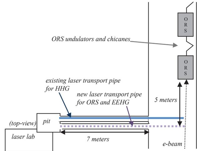
Figure 3: Location of new laser transport line with respect to the accelerator tunnel, laser table and first ORS undulator.
