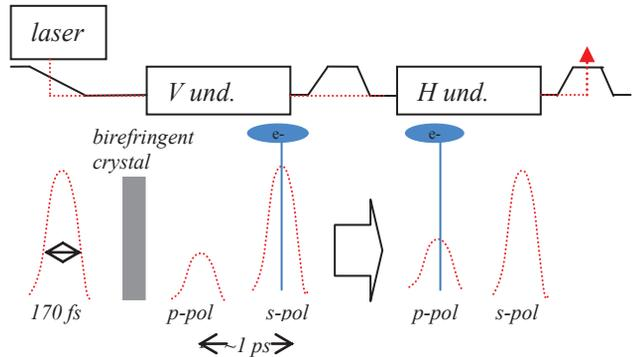
Figure 5: Generating a delay between *s* and *p* polarization so that the pulse can be used to seed in both undulators. The undulator labeled *H und.* produces horizontal oscillations and *V und.* produces vertical oscillations.
