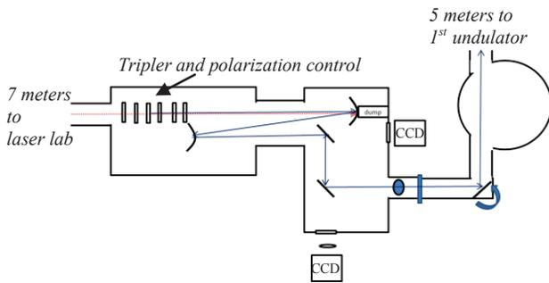
Figure 4: Layout of optics in the accelerator tunnel. Frequency tripler and polarization control optics are followed by a Galilean telescope and four motorized steering mirrors. A window sits between the last two mirrors.
