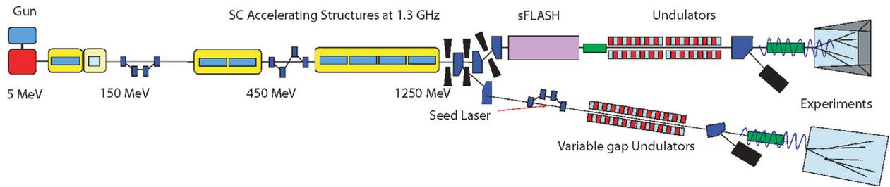
Figure 1: Schematic layout of the FLASH facility. The electron gun is on the left, the experimental hall on the right. Behind the last accelerating module, the beam is switched between FLASH1, which is the present undulator line, and FLASH2, which is the upgrade. Behind the extraction point, space is reserved for an additional laser system for seeding.
