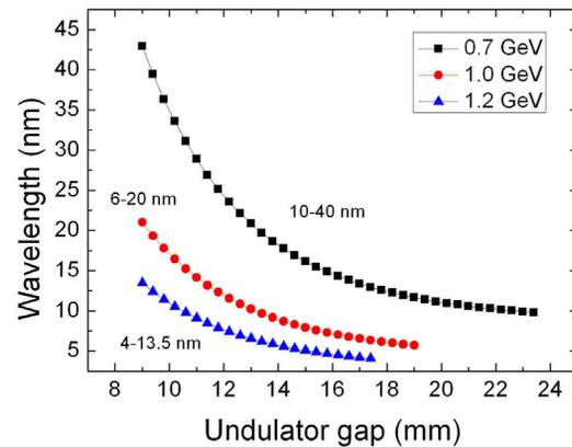
Figure 2: Wavelength range which can be reached for three different energies that are mostly used at FLASH.
