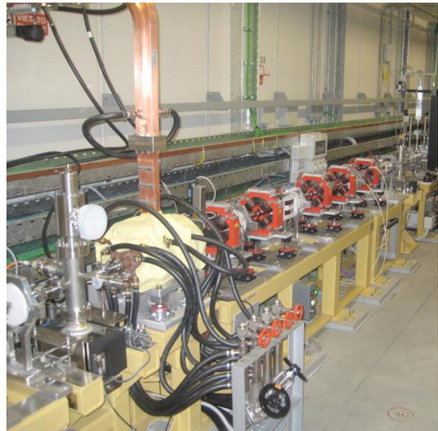
Figure 1: The low energy deflector in the FERMI@Elettra Linac.
