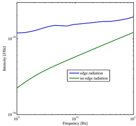
Figure 2: Spectral dependence of the radiation emitted from the last dipole of BC1. The blue curve includes velocity term that dominated for edge radiation while the green is classical synchrotron radiation.
