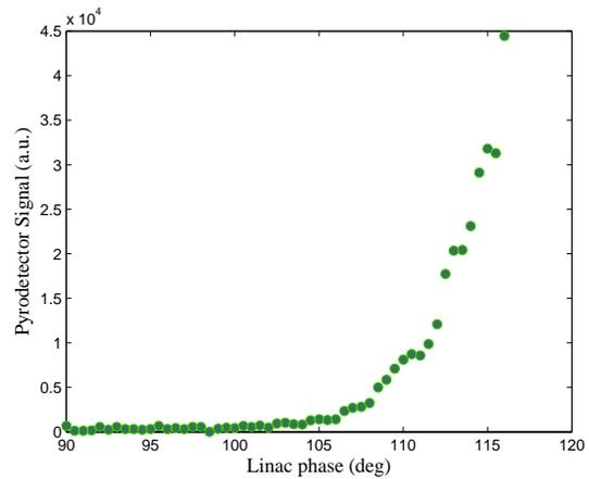
Figure 7: Pyrodetector signal vs linac 1 phase.
