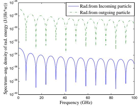
Figure 4: Spectrum-angular density of the energy radiated by a 250 MeV charge entering and going out from a semi-infinite waveguide versus frequency, at an angle  $\theta$  of  $\pi/2$  rads from the pipe axis.
