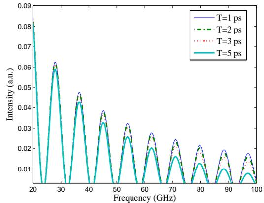
Figure 5: Spectrum-angular density of energy radiated by a rectangular electron bunch passing through a gap in a waveguide, calculated for different bunch lengths, and for a bunch energy of 250 MeV. The density has been calculated at an angle  $\theta$  of  $\pi/2$  rads from the pipe axis.
