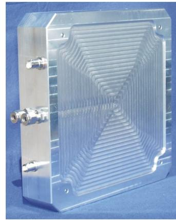
Figure 5: Photo of the ionization chamber.
