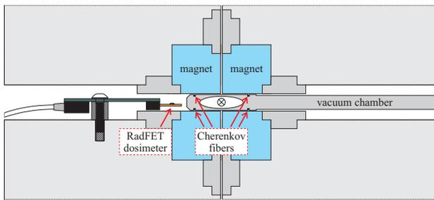
Figure 4: Cross section of an FEL-1 undulator with closed gap. The positions of the four Cherenkov fibers and of a RadFET dosimeter are indicated.
