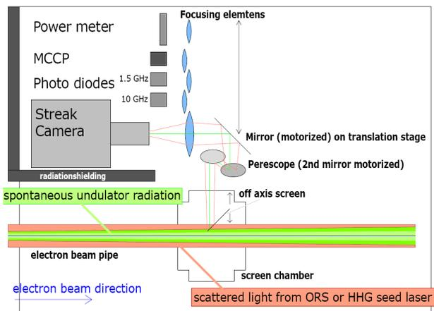
Figure 2: Planned layout for the diagnostics on one of the optical stations. Undulator radiation and laser light will be reflected by on off axis screen
