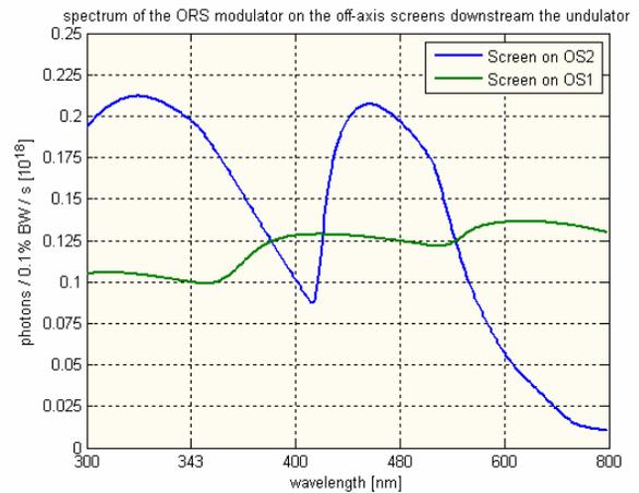
Figure 4: Photon flux on the two screen 2.4 m and 7.3 m after the ORS modulator.
