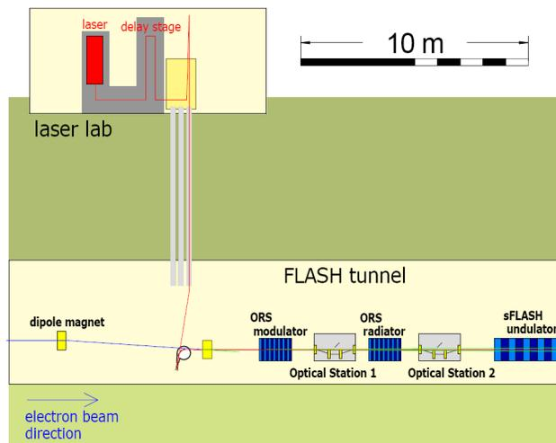
Figure 1: ORS and sFLASH section of FLASH
