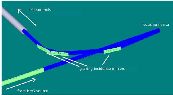
Figure 3: Part of the ZEMAX model of the HHG laser transfer line
