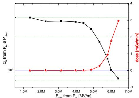
Figure 6: Quality factor  $Q_0$  versus acceleration gradient.
