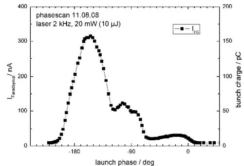
Figure 12: Schottky scan at 2 kHz and 20 mW.
