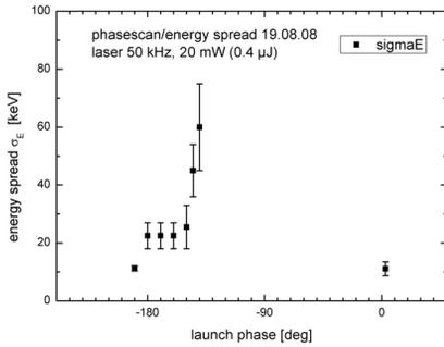
Figure 14: The rms energy spread as function of laser phase.
