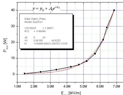
Figure 5: RF power dissipation vs. gradient.
