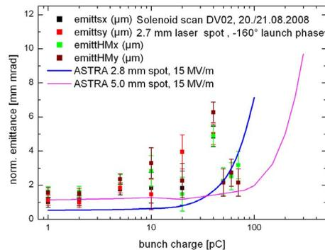
Figure 16: Normalized transverse emittance as function of bunch charge for  $-160^\circ$  laser phase and 2.7 mm laser spot, as well as comparison with ASTRA simulation (15 MV/m peak field, 2.8 mm and 5 mm circular flat top laser spot, optimized phase and cathode position).
