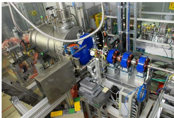
Figure 2 : Photograph of the SRF gun in the ELBE accelerator hall.
