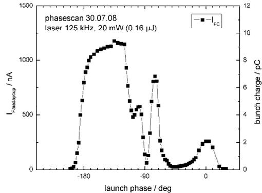
Figure 11: Schottky scan at 125 kHz and 20 mW.
