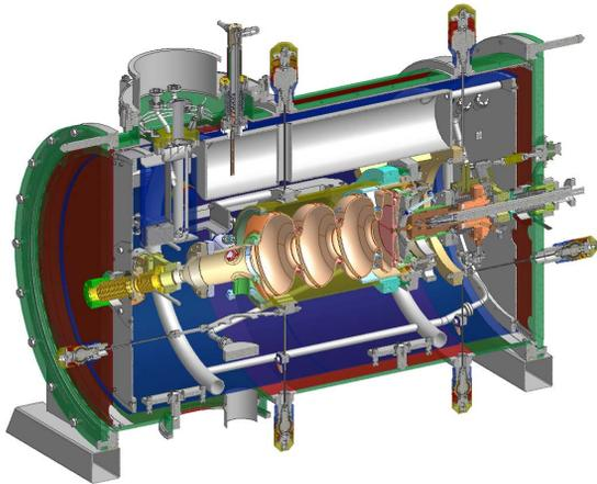
Figure 1: Design of the SRF Gun cryomodule.
