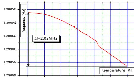
Figure 4: Cool-down curve showing the cavity resonance frequency versus temperature.
