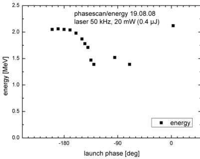
Figure 13: Energy as a function of laser phase.
