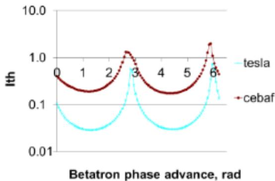
Figure 3: BBU threshold currents for two different types of accelerating cavities and different amount of betatron phase advance [8].
