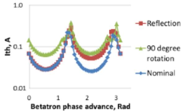
Figure 4: BBU threshold currents for different amount of betatron phase advance and coupled motion of x and y planes in tranverse phase space using reflectors (skew quadrupoles) or solenoids [8].
