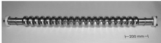
Figure 2: S-DALINAC 20 cell cavity.
