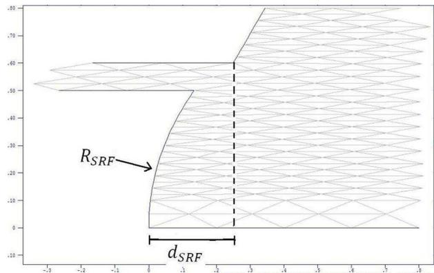
Figure 8: Close-up of the photocathode from Figure 7 with the definitions of the parameters  $d_{SRF}$  and  $R_{SRF}$  illustrated.
