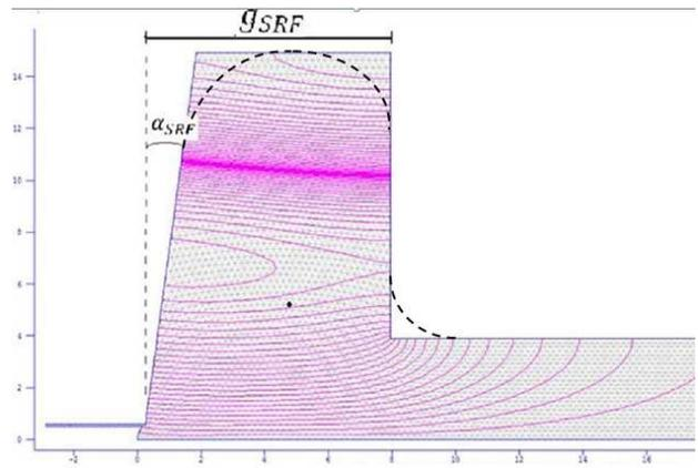
Figure 7: Simplified SRF gun geometry, shown in the  $z$ - $r$  plane, with the definitions of the parameters  $\alpha_{SRF}$  and  $g_{SRF}$  illustrated. The axes here are reversed from those used for the DC gun in Figures 2: the horizontal axis is the beamline  $z$ ; the vertical axis is that of the cylindrical coordinate  $r$ . Lines of constant  $rH_\phi$ , where  $H_\phi$  is the magnitude of the azimuthal component of the magnetic field are shown.
