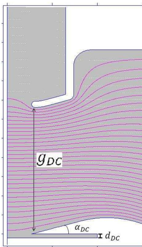
Figure 2: Closeup of the DC gun geometry, shown in the  $z$ - $r$  plane, with the definitions of geometry parameters  $\alpha_{DC}$ ,  $g_{DC}$ , and  $d_{DC}$  illustrated. The vertical axis is the beamline  $z$ ; the horizontal axis is that of the cylindrical coordinate  $r$ . Equipotential lines are shown.
