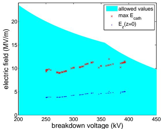
Figure 4: Simulation data from the DC gun optimization overlaid on the graph of maximum electric field as a function of breakdown voltage.  $\max E_{cath}$  is the maximum electric field at the cathode electrode allowed under the breakdown constraint.  $E_z(z=0)$  is the electric field at the cathode chosen by the optimizer.
