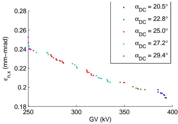
Figure 5: The resulting optimal front from the DC gun optimization after 254 generations, with each solution colored by its respective  $\alpha_{DC}$ . The electron beam is represented with 28,000 macroparticles.
