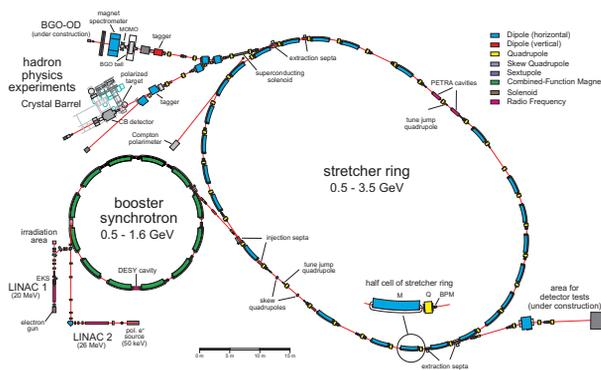
Figure 1: The electron stretcher accelerator ELSA.
