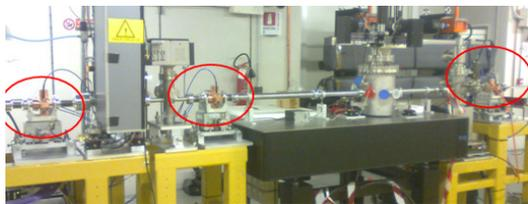
Figure 5: The first three Cavity BPMs in the spreader section.
