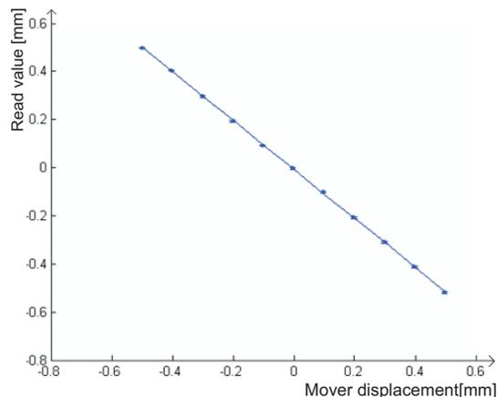
Figure 3: Calibration of the Cavity BPM.
