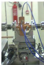
Figure 2: The Cavity BPM with the dedicated mover.
