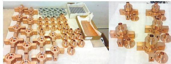
Figure 1: Parts of the Cavity BPM, before brazing
