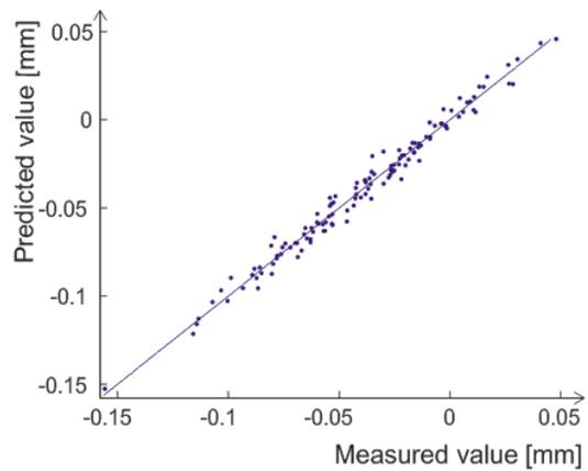
Figure 6: Plot of the predicted-measured values of the electron beam position.
