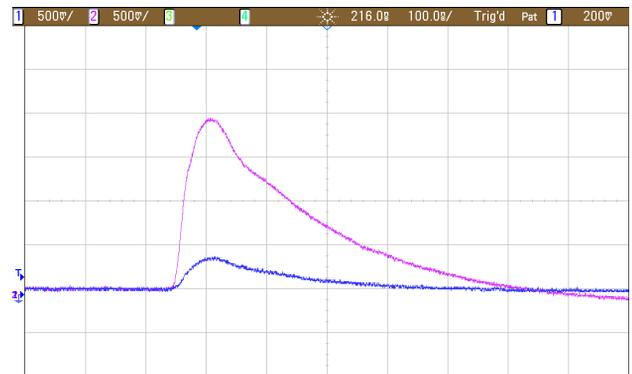
Figure 4: C-BPM X axis envelope signals with 50pC off axis Beam. Ch1: envelope Σ signal, Ch2: envelope Δ signal.
