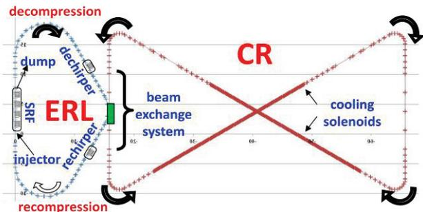
Figure 1: A schematic drawing of an ERL-circulator ring based electron cooling facility.
