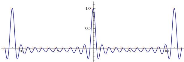
Figure 3. The RF waveform that results in a kick to every eleventh bunch with the other bunches receiving no kick.
