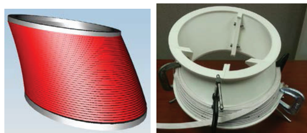
Figure 7: Conceptual drawing (left) and 3d printer version (right) of the Nb 3 Sn HS spool and conductor that will be fabricated and tested in the Fermilab Vertical Magnet Test Facility. The test will use two layers of cable.
