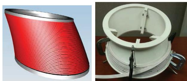
Figure 7: Conceptual drawing (left) and 3d printer version (right) of the Nb<sub>3</sub>Sn HS spool and conductor that will be fabricated and tested in the Fermilab Vertical Magnet Test Facility. The test will use two layers of cable.
