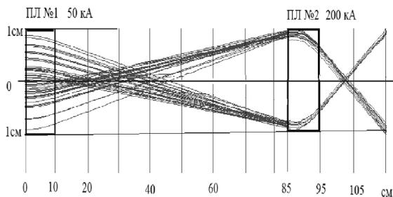
Figure 9: Formation a converging conic beam by means of two plasma lens.
