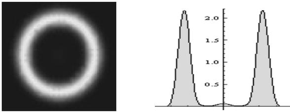
Figure 8: The light output from a scintillator and the distribution of ion  $Fe^{+26}$  density calculated in the model approximation for the experimental condition.
