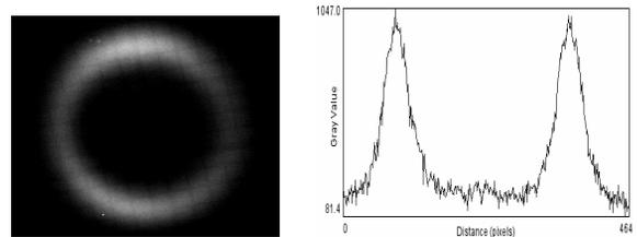
Figure 6: Light output from scintillator and the density distribution of ion  $Fe^{+26}$  at 1.7  $\mu s$  after beginning of discharge at distances of 30 cm for current of 150 kA. The ring diameter is 9 mm.
