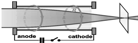
Figure 1: Ion focusing in a plasma lens.
