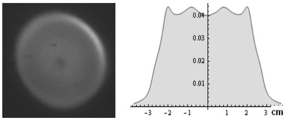
Figure 4: The light output from the scintillator and the density distribution of the ion  $C^{+6}$  at 8.5  $\mu s$  after beginning of discharge at distances of 110 cm for current of 80 kA. The spot rms diameter is 40 mm.
