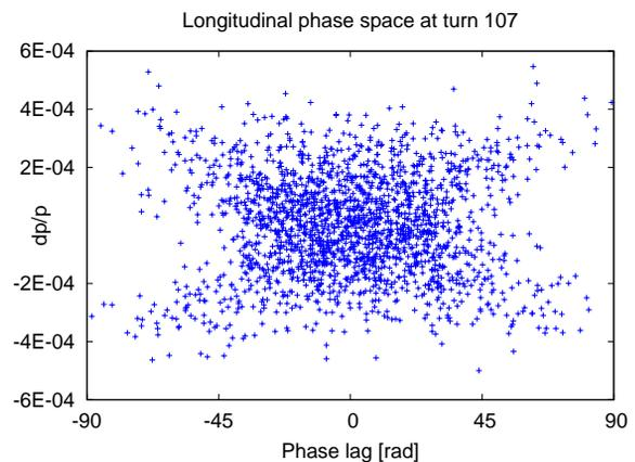
Figure 4: Longitudinal phase space plot at the end of the capture process with 202 MHz, with a 300 ns long barrier bucket. A starting  $dp/p = 7 \times 10^{-5}$  was assumed. This is a simulation result including longitudinal space charge forces.
