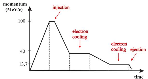
Figure 6: Schematic view of ELENA cycle.
