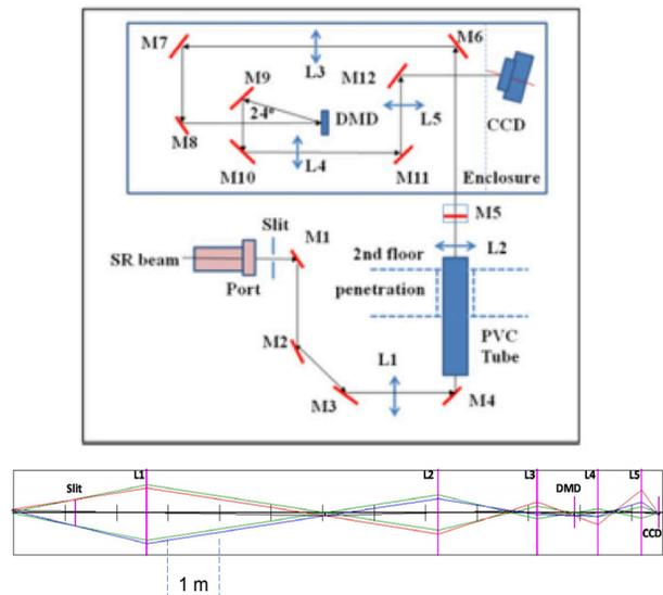
Figure 1: (top) layout of the optical transport showing mirrors (M) and lenses (L); (bottom) ray tracing diagram.
