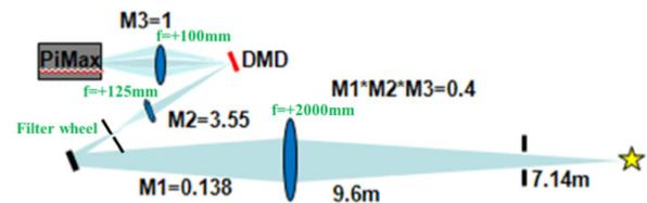
Figure 4: Optical imaging system at SPEAR3.
