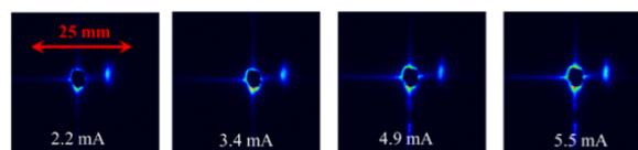
Figure 7: Fixed turn images of injected beam with stored beam blocked by intensity threshold masks for different stored beam currents.
