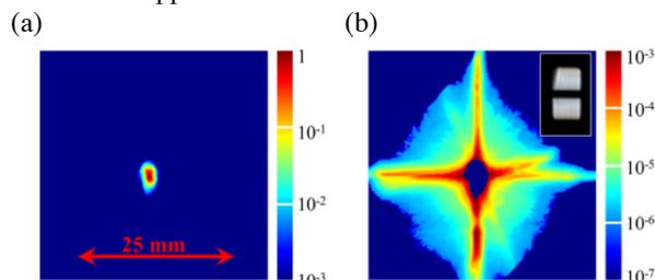
Figure 5: Log normalized intensity profile of the SPEAR3 stored beam; (a) first 3 decades; (b) last 4 decades and insert showing aperture function of the visible beam line.
