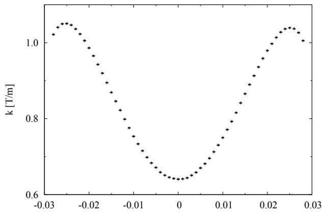
Figure 2: Quadrupole field gradient on the x-axis
