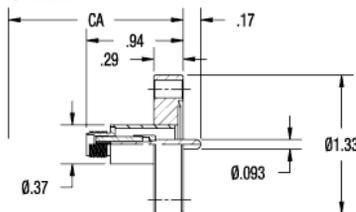
Fig. 4: Conflat flange with SMA coaxial feedthrough. Shown here is a possible model by MDC Vacuum Products. Dimensions in inches.
