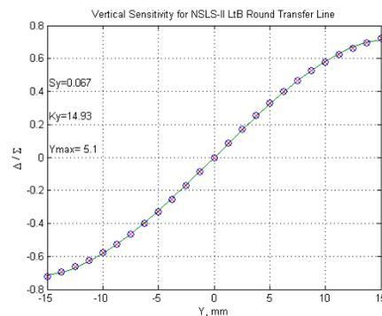
Fig. 6: Horizontal (top) and vertical (bottom) beam motion sensitivity for the round chamber. These figures have sensitivity numbers (Sxy), coefficients for calculating position from the measured BPM button voltages (Kxy), and limits where linearity drops by 10% from the central region. With centered beam, each button intercepts 12.4% of a passing charge.
