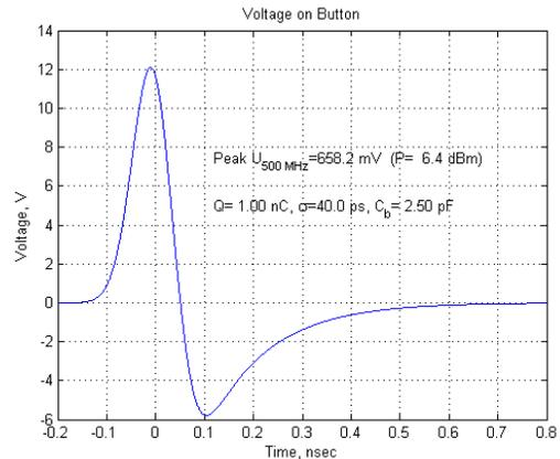
Fig. 9: Signal induced by a centered single bunch with 40 ps (rms) length and 1 nc charge on a button in the elliptical chamber.
