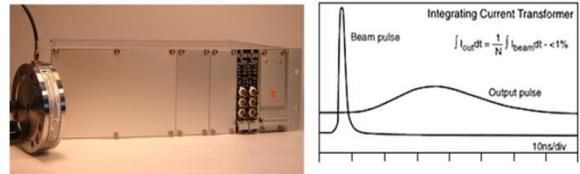
Figure 3. Integrating current transformer (ICT).
