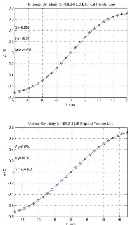
Fig. 8: Horizontal (top) and vertical (bottom) beam motion sensitivity for the elliptical chamber.
