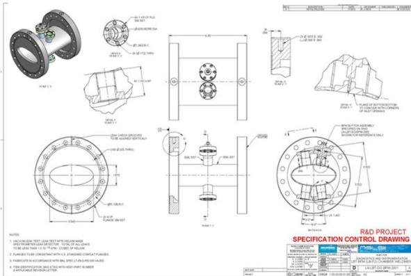
Figure 7: Elliptical (40 x 90 mm) chamber assembly.
