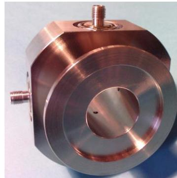
Figure 5: BAM 4-electrode (open coax-line type) pick up.
